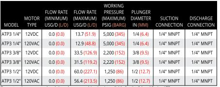
Flow rates shown are per head. Any plunger combination is available for the 2-head Series ATP. Motor Type 12VDC = Variable Speed 6-67 RPM Motor, Class 1 Division 2
