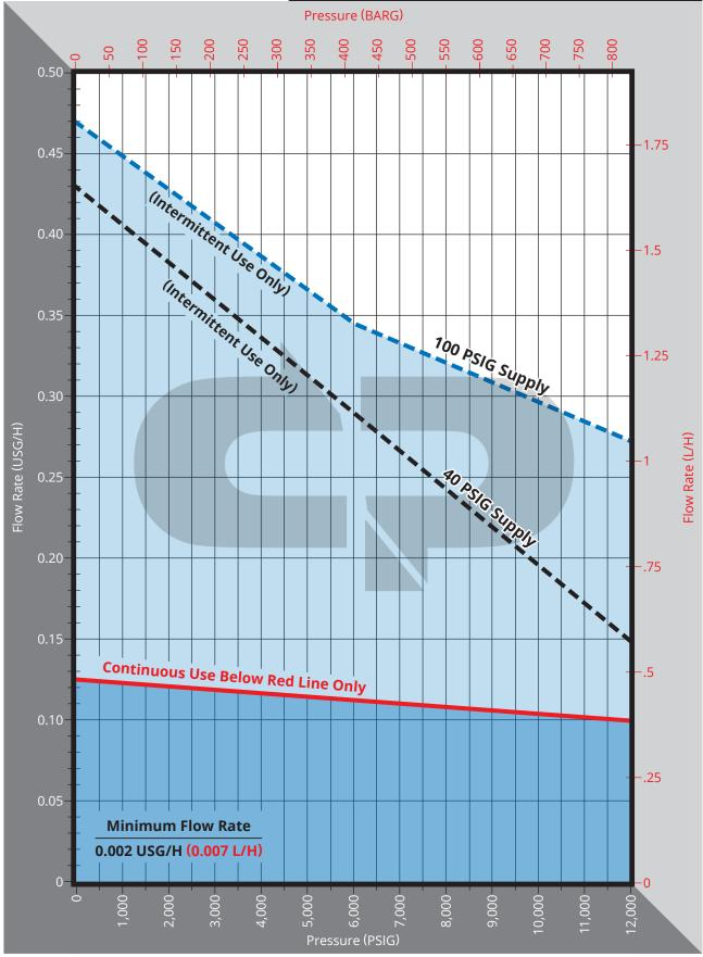
Maximum Pressure: 12,000 PSIG Metallic Head / 300 PSIG PVC Head. This performance curve should be used to select an appropriate model. It was generated with empirical data and supersedes calculated or theoretical table data. High pressure model pump heads are dedicated and do not accept other size plungers. DOC1250 High Pressure .125FCP1 USGH REV22
