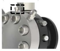
NOTE: If the pump is not new, it is possible for dried or solidified chemical to be present in the bleed and check valve assemblies. If your pump does not bleed when following the directions above, try cleaning these items in solvent and replacing them.
