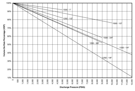
3.2.2.2 Volume per stroke decreases as the discharge pressure rises. It is necessary to apply a Volume De-Rating Percentage (VDP) to the Unrated Stroke Rate (USR). The VDP is based on the expected discharge pressure the pump will experience. Use the VDP Graph (Figure 5) to find the VDP, taking care to use the curve for your specific plunger diameter:
