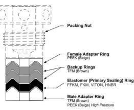
NOTE: When replacing adjustable packing, always install the packing rings exactly as they are shipped. Rearranging the order of the vee-rings in an adjustable packing set will reduce the life of the elastomer ring in the packing set.
