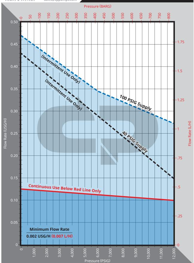
Maximum Pressure: 12,000 PSIG Metallic Head / 300 PSIG PVC Head. This performance curve should be used to select an appropriate model. It was generated with empirical data and supersedes calculated or theoretical table data. High pressure model pump heads are dedicated and do not accept other size plungers.
