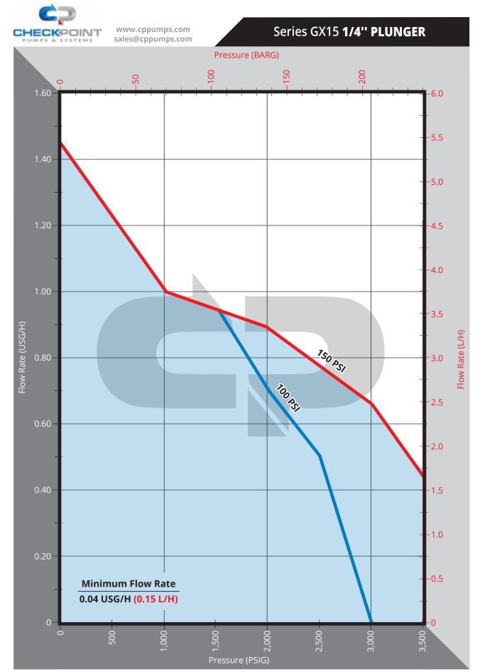
Maximum Pressure: 3,500 PSIG. This performance curve was generated with empirical data, supersedes calculated or theoretical table data, and should be used to select an appropriate model. This model features a modular head design that allows interchangeability with other plunger sizes with the appropriate parts.
