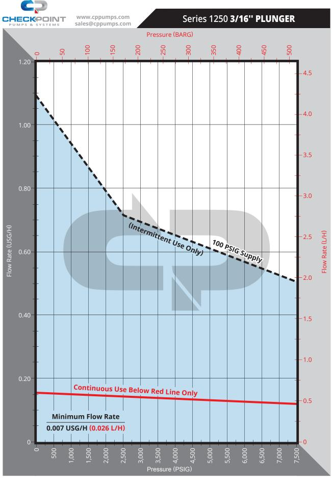
Maximum Pressure: 7,500 PSIG Metallic Head / 300 PSIG PVC Head. This performance curve was generated with empirical data, supersedes calculated or theoretical table data, and should be used to select an appropriate model. The metallic head version of this model features a modular head design that allows interchangeability with other plunger sizes with the appropriate parts.
