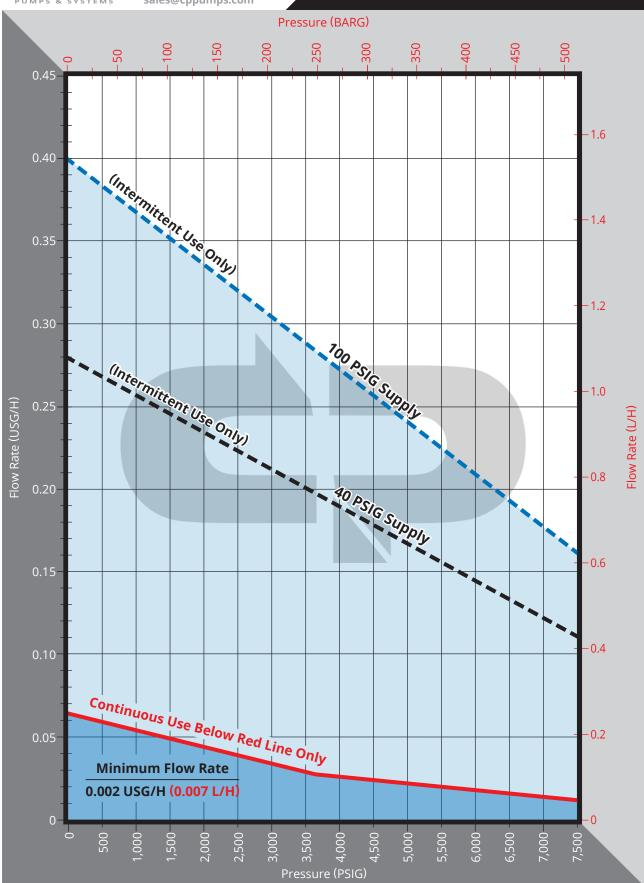
Maximum Pressure: 7,500 PSIG Metallic Head / 300 PSIG PVC Head. This performance curve was generated with empirical data, supersedes calculated or theoretical table data, and should be used to select an appropriate model. The metallic head version of this model features a modular head design that allows interchangeability with other plunger sizes with the appropriate parts.
