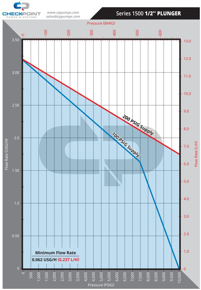
Maximum Pressure: 10,000 PSIG Metallic Head / 300 PSIG PVC Head. This performance curve was generated with empirical data, supersedes calculated or theoretical table data, and should be used to select an appropriate model. The metallic head version of this model features a modular head design that allows interchangeability with other plunger sizes with the appropriate parts.
