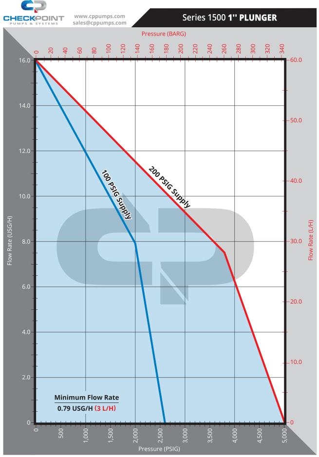
Maximum Pressure: 5,000 PSIG Metallic Head / 300 PSIG PVC Head. This performance curve was generated with empirical data, supersedes calculated or theoretical table data, and should be used to select an appropriate model. The metallic head version of this model features a modular head design that allows interchangeability with other plunger sizes with the appropriate parts.
