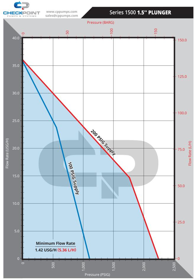
Maximum Pressure: 2,250 PSIG. This performance curve was generated with empirical data, supersedes calculated or theoretical table data, and should be used to select an appropriate model. The 1.5" model pump head is dedicated and does not accept other size plungers. DOC1500 1.5FCP1 USGH REV11
