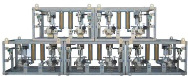
A solution by CheckPoint Pumps and Systems was supplied to tackle the daunting obstacles facing Champion-Petrobras. These units were to be located in the FPSO's turret, which have a very constrained design footprint. H<sub>2</sub>S scavenger was to replace paraffin inhibitor, and it was required that ten different injection points be supplied by ten pumps. These pumps were to supply chemical at the rate of 100 LPH (24 GPH) against pressures of up to 185 kg / cm² (2700 PSIG).
